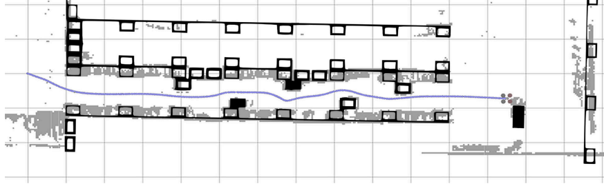
Figure 24: One of our runs for the slalom task. In black we show the actual obstacle course layout. The hollow obstacles in the aisle are similar to the tower shown in Figure 23 while the filled black ones are scissor lifts. The gray regions are the projection of map created by the robot onto the 2D plane. The robot starts near the opening on the left and has to reach the target represented by the black rectangle on the right. The path of the robot shows it moving in a zigzag fashion in order to avoid the obstacles. Each grid cell is 5\text{ m} \times 5\text{ m} .
