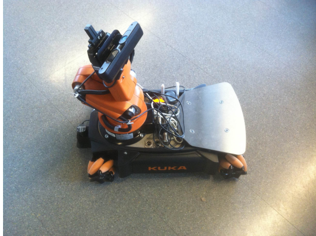
Figure 5.5: KUKA youBot mobile manipulation platform. Equipped with ASUS Xtion Pro Live RGB-D camera mounted at the wrist of the manipulator arm, and Hokuyo URG-04LX-UG01 laser scanner mounted on the front bumper.
